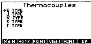
As an example, suppose you want to find the corresponding temperature of an E type thermocouple showing a 22.13 millivolt reading. First, move the pointer to TYPE E and press **ENTER** to display the following screen:
