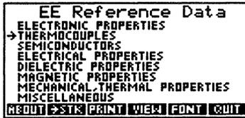
This analysis tool is designed to convert a temperature to a thermocouple output in millivolts and vice versa. The software has the ability to handle T, E, J, K and S type thermocouples. The implied assumption for a reference temperature is 0 °C. The thermocouple computations are based on the IPTS-68 standards.
