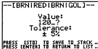
The result is presented as a 120\_?, along with tolerance value, the color scheme for a standard resistor. The standard values work with capacitors and inductors in addition to resistors.
