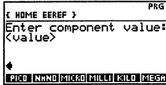
When entering a component value, a row of softkeys PICO, NANO, MICRO, MILLI, KILO, MEGA, FEMT, GIGA enhance data entry by adding appropriate multipliers.
