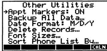
There are six Utility functions available. To select a Utility, use the **▲** and **▼** keys to move the arrow to select the desired Utility and press **ENTER**.
