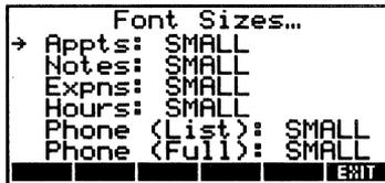
To change a font size, move the arrow to the appropriate name and press **ENTER**. This will toggle the display font between the LARGE and SMALL font (the report font always remains large). Press **EXIT** to return to the Utilities screen.
